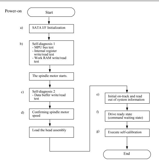
Figure 4.3 Power-on operation sequence
